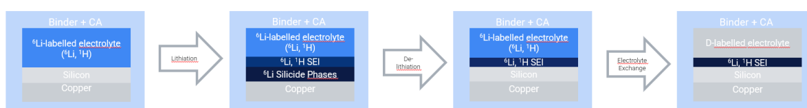
Figure 2 Exemplary electrolyte exchange methodology for silicon. Attenuating phases are marked in blue, while phases invisible to neutron radiation are depicted in grey.
