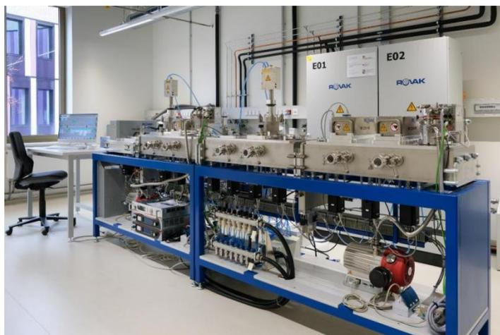
**Fig. 1:** Sputter-FLA system for thin film sample preparation for the OPINCHARGE project.
